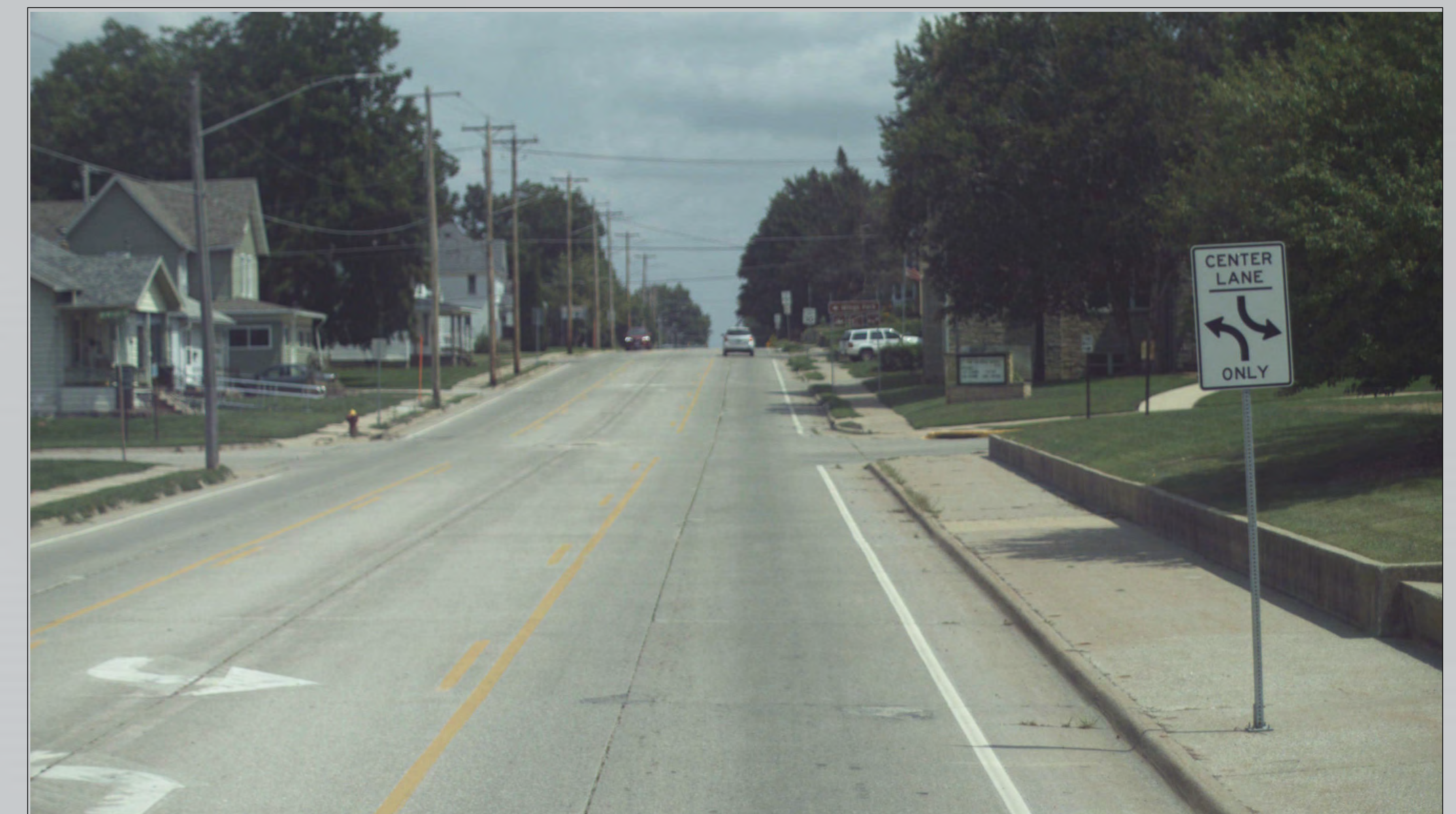
Example of Center Two-Way Left-Turn Lanes (TWLTL) in Oelwein, Iowa.
