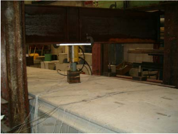
Figure 56 – Deck Panel Testing
