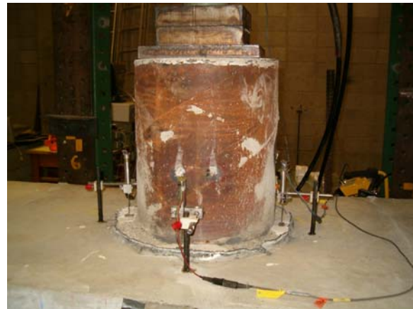
Figure 55 – Loading Pipe Pile
